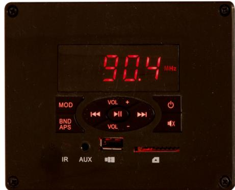
Aux, USB, SD card to connect with different devices to play MP3 files.
